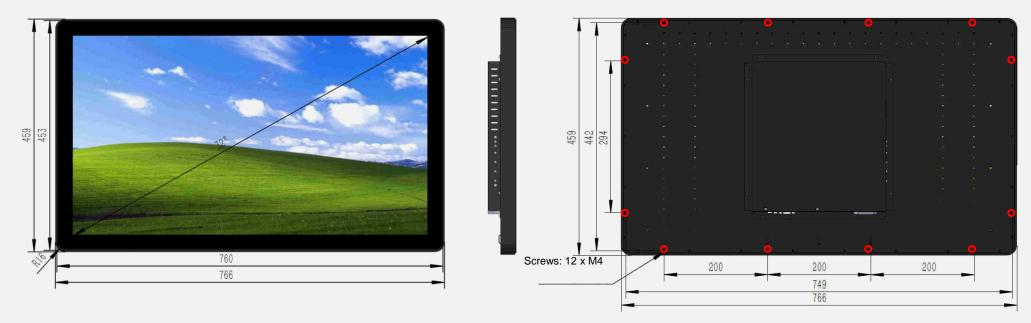
Screw hole spec: 12 x M4 10mm lenght, pitch: 0.7.
